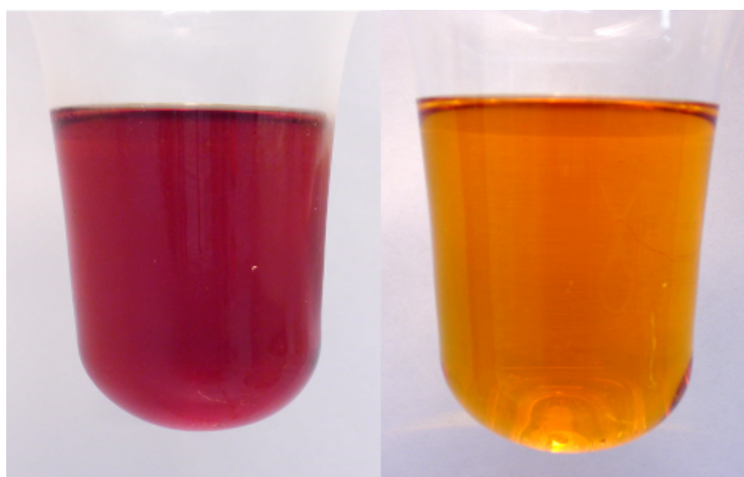
Fig. S1. Solution of [\text{FeL}(\text{NCS})_2] ( 1 ) in acetone just above the melting point (left) and at room temperature (right).
